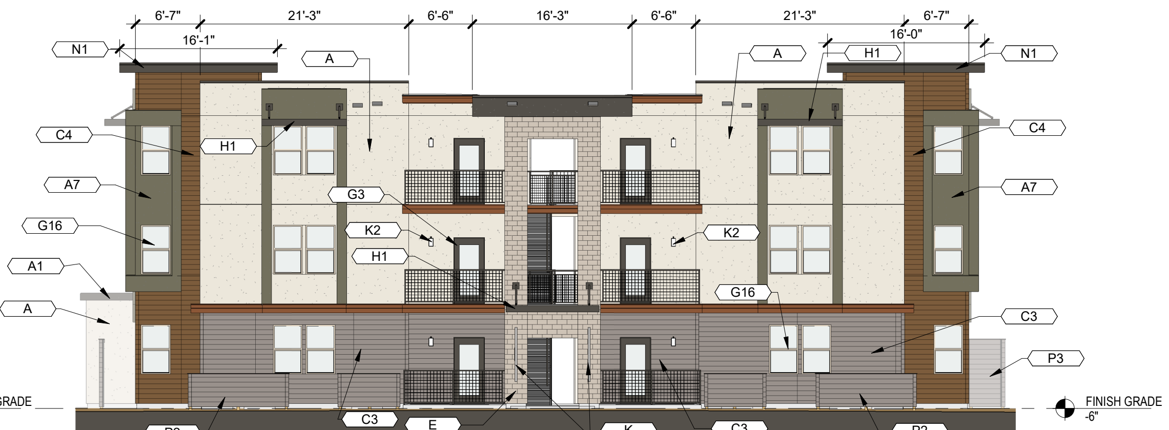
3 12 UNIT BUILDING - REAR ELEVATION SCALE: 1" = 10'-0"
