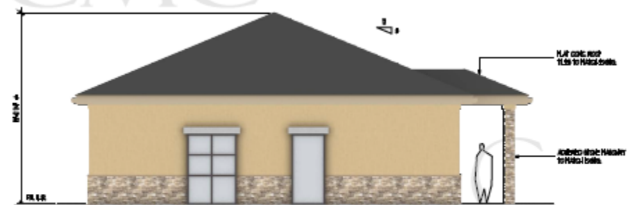
SIDE BUILDING ELEVATION (WEST) SCALE 3/8" = 1'-0"
