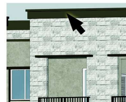
11. CORNICE CAPS TO MATCH PAINT SPEC C
