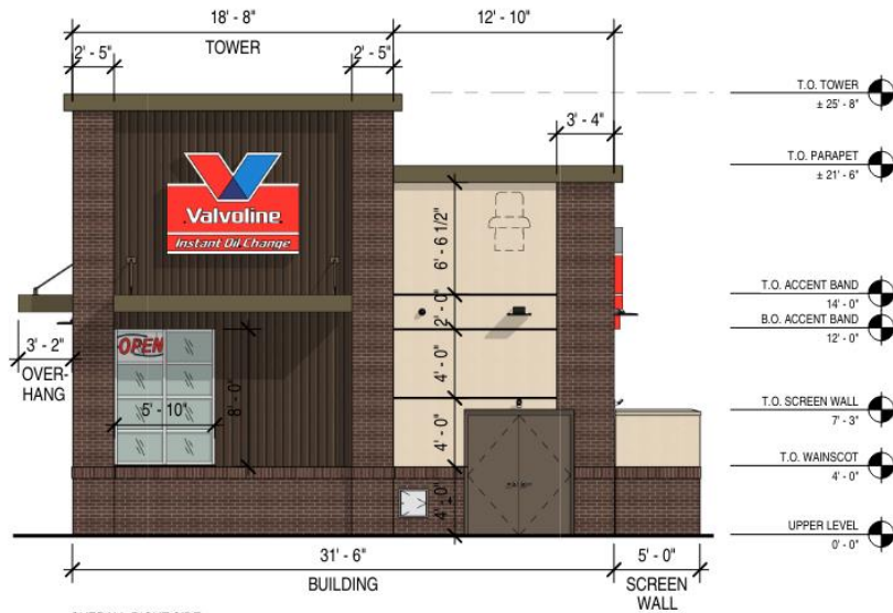
2 OVERALL RIGHT SIDE EXTERIOR ELEVATION (RIGHT) Scale: 1/8" = 1'-0"
