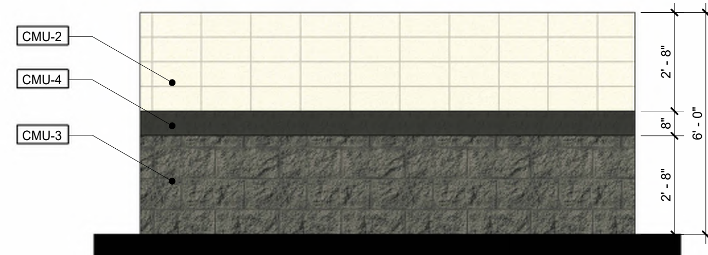
4 REFUSE ENCLOSURE BACK ELEVATION 3/8" = 1'-0"
