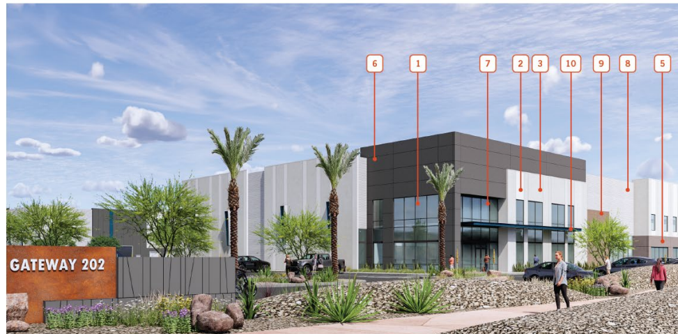
9 CMU BLOCK: COLOR/FINISH: MERLOT / SPLIT FACE (OR APPROVED EQUIVALENT MATERIAL WITH COMPARABLE COLOR AND TEXTURE, SUCH AS FORMLINER)
