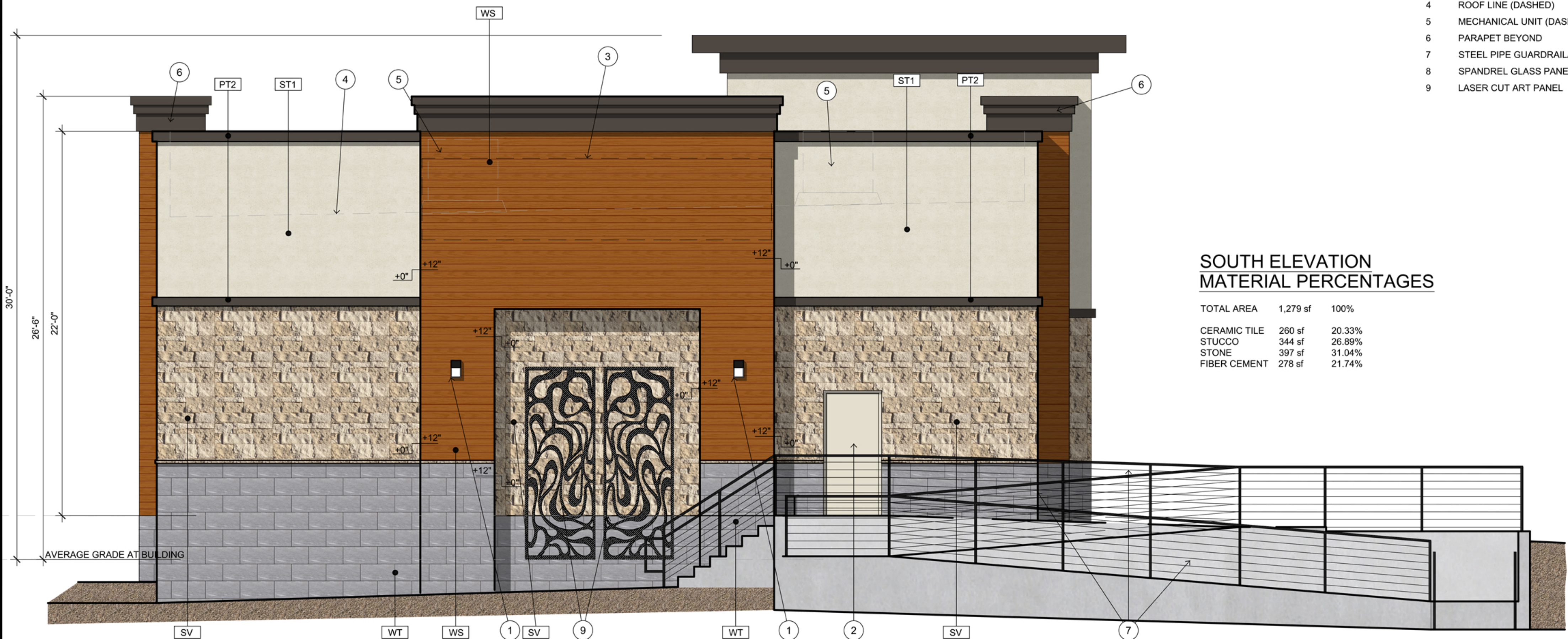
2 EXTERIOR ELEVATION - SOUTH
