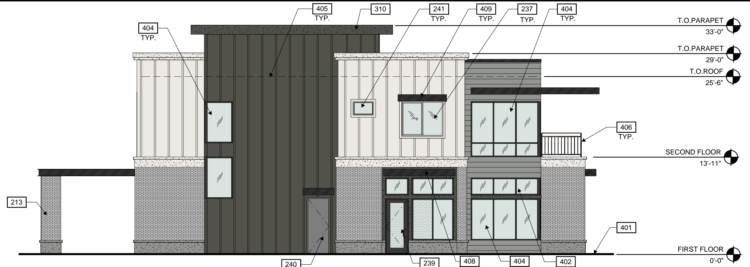
MIXED USE BUILDING - WEST EXTERIOR ELEVATION ④
