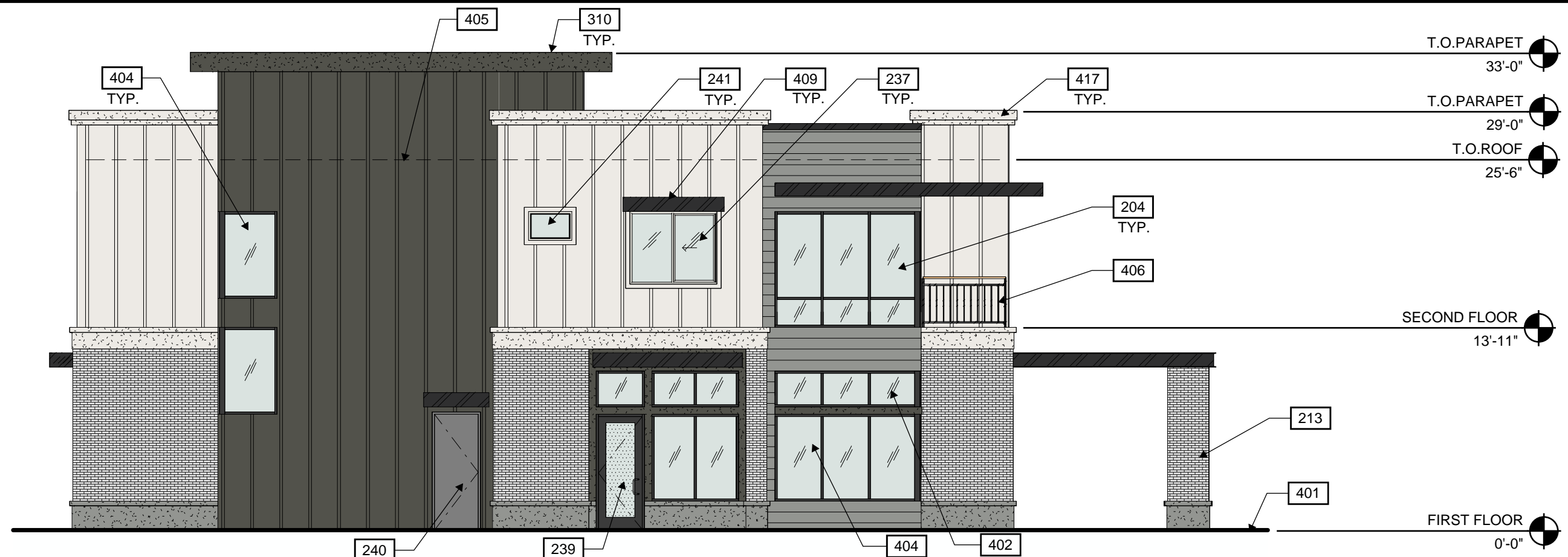
MIXED USE BUILDING - EAST EXTERIOR ELEVATION ②
