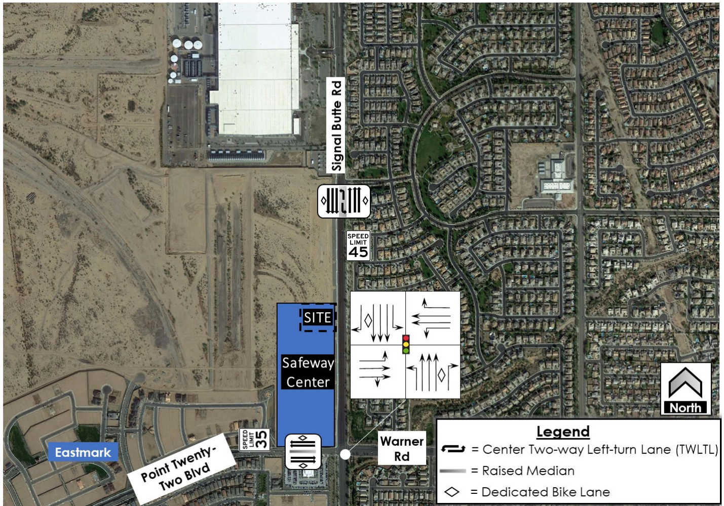
Figure 2: Existing Lane Configuration and Stop Control
