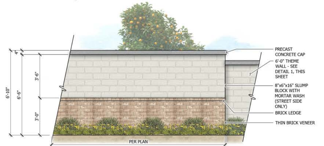
3 2'-0" View Fence over 4'-0" CMU Wall SCALE: 1/2"=1'-0"
