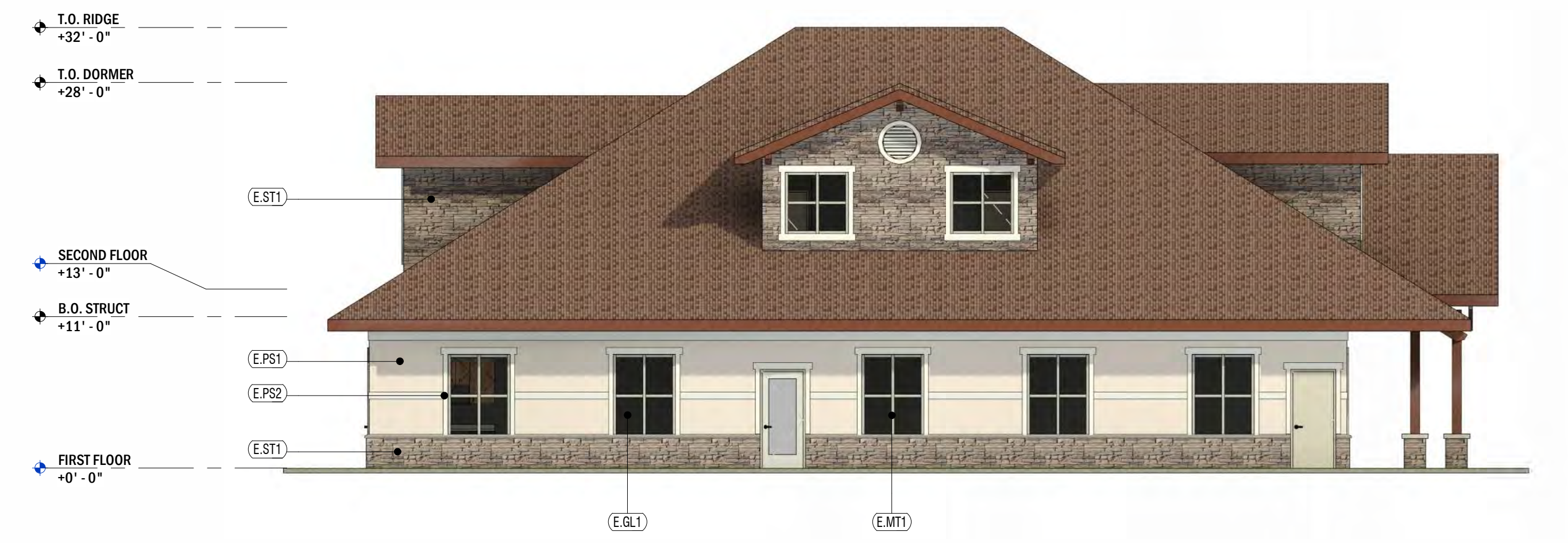
4 REAR (NORTH) ELEVATION 1/8" = 1'-0"
