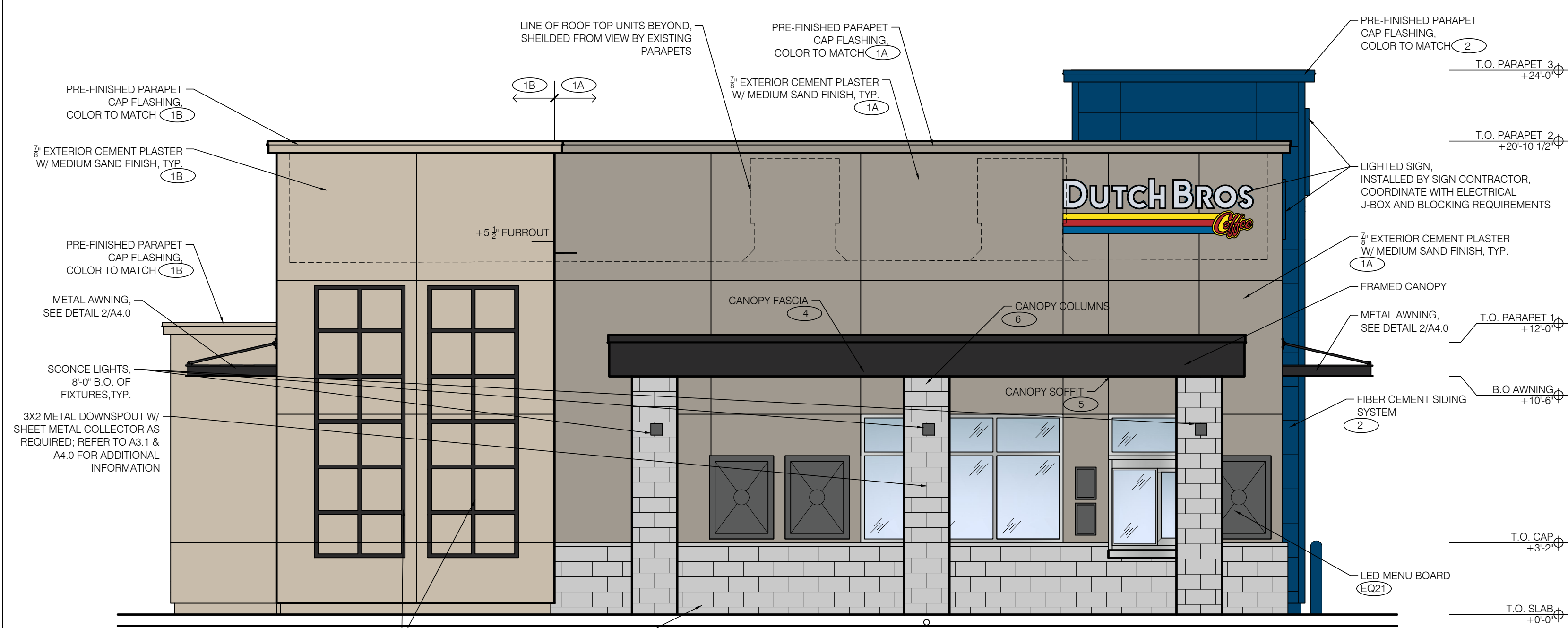
2 EAST ELEVATION - WALK-UP WINDOW SCALE: 1/4" = 1'-0"
