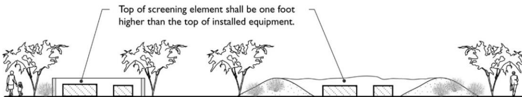
FIGURE 11-30-9.A.(2): SCREENING OF GROUND-MOUNTED EQUIPMENT
