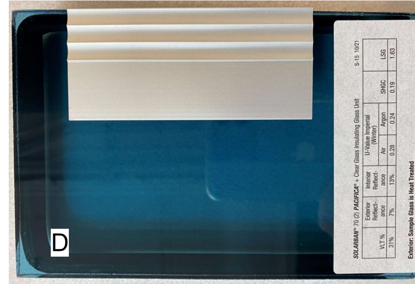
STOREFRONT SYSTEM: 1" INSULATED GLAZING, VIBRO "PACIFICA AND SOLARBAN 70" WITH CLEAR ANODIZED ALUMINUM FRAME
