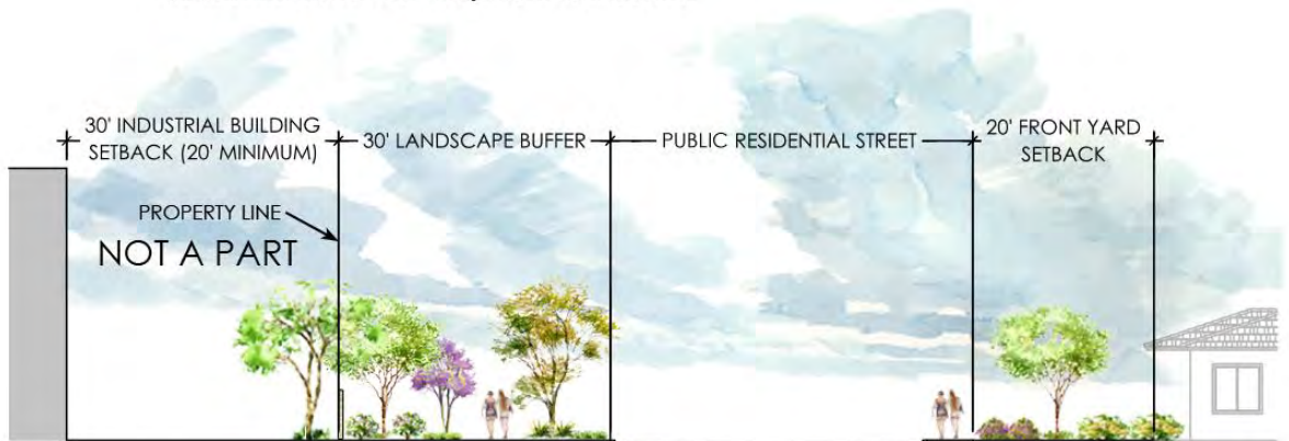
Section A - Front Yard Residential Buffer Section Adjacent to Industrial
