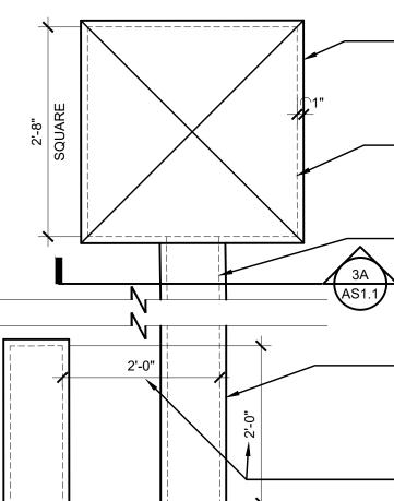
CONCRETE MASONRY SOLID CAP. SPLIT-FACE, OVER COLUMN WITH MIN. 1" OVERHANG. PAINTED (EP-01). SLOPE FOR POSITIVE DRAINAGE.
