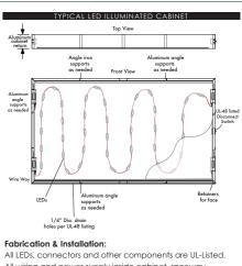
All wiring and power supply inside cabinet, raceway or conduit as needed. Type 1, un-braced construction. External disconnect switch. Primary power supplied by others
