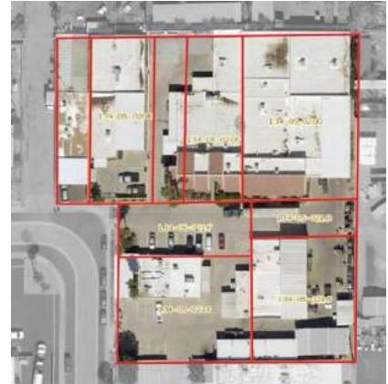
Parcels were subdivided in such a way that does not provide any street frontage or sufficient access to a public roadway.
