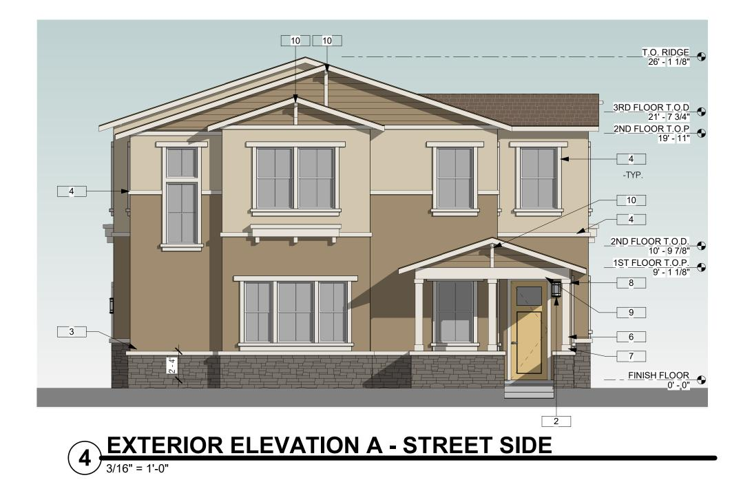
T.O. RIDGE 26' - 1 1/8" 3RD FLOOR T.O.D 21' - 7 3/4" 2ND FLOOR T.O.P 19' - 11" -TYP. 4 2ND FLOOR T.O.D. 10' - 9 7/8" 1ST FLOOR T.O.P. 9' - 1 1/8" \_\_\_\_3\_\_\_ FINISH FLOOR 0' - 0"
