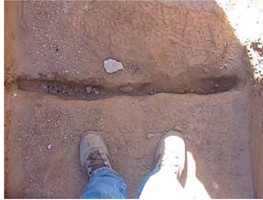
Photo 2: The primary earth fissure F4 is exposed across the bottom of the trench. The Earth fissure crack, about 0.15 ft. to 0.25 ft. wide, was found in caliche cemented soil below the fill and is filled with brown, fine silty sand with gravel. The fissure gully and fissure fill bridges open fissure crack about 5.5 ft. bgs. The earth fissure bearing is N68°W.
