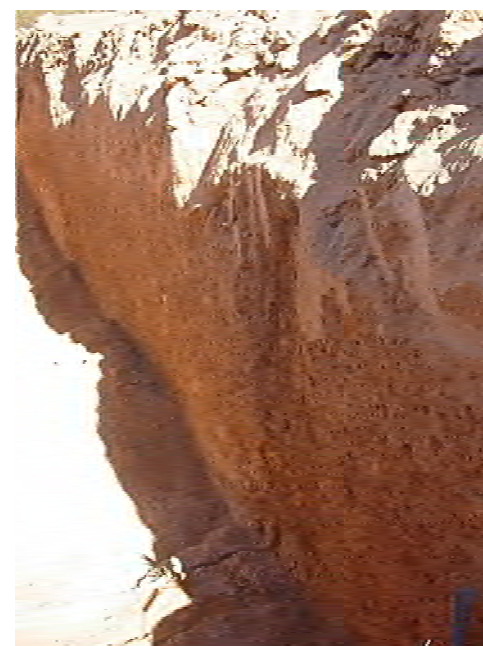
Photo 4: Soil profile adjacent to the F5 fissure cracks in east wall of Trench 3:
