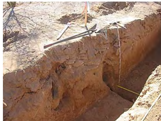
Photo 3: Earth Fissure F3 exposed in east wall and bottom of trench wall. Width of fissure gully rubble backfill zone about 10 ft. wide along parallel to trench wall. Several lateral to sublateral, partially fill erosion pipes exposed in trench wall. Fissure azimuth is N65°W.
