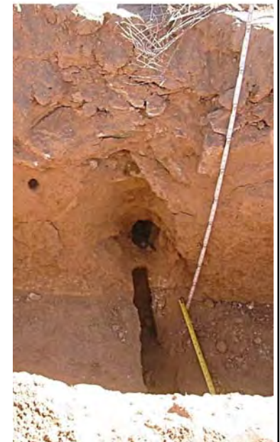
Photo 4: Soil profile adjacent to fissure crack in east trench wall:
