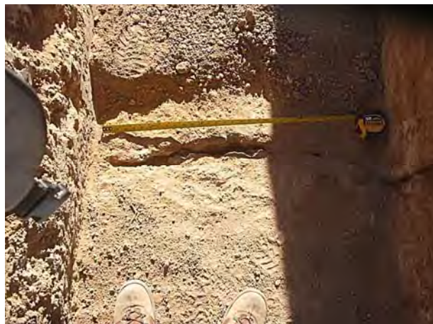
Photo 2: Earth fissure F6 is exposed across the bottom of the trench. The earth fissure crack, about 0.45ft. to 0.9 ft. wide, was found in caliche cemented soil below the overburden soil. The gully fill is with light brown, silty coarse sand mixed with trash and asphaltic concrete rubble. The fissure fill bridges open fissure crack to more than 5 ft. bgs.
