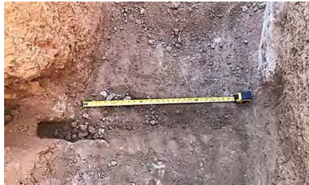
Photo 2: Earth Fissure F3 crack exposed across the bottom of the trench. The crack was found in caliche cemented soil about 0.4 feet wide and is filled with a brown silty sand with small fill debris. Fill bridges open fissure crack about 6.5 ft. bgs. Fissure bearing is N86°W.
