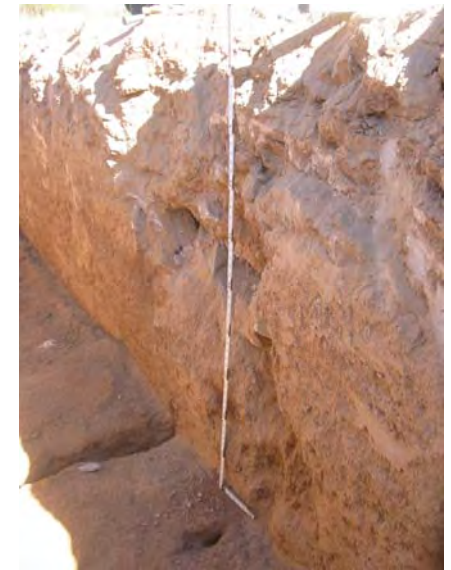
Photo 4: Soil profile adjacent to the F4 fissure cracks in east wall of Trench 2:
