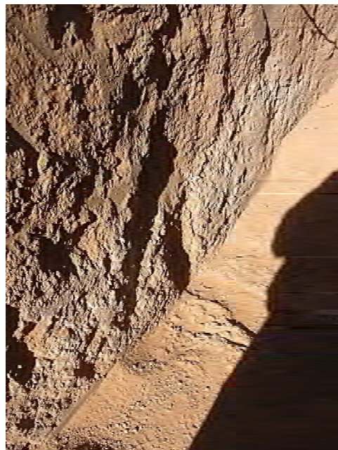
Photo 2: View of west trench wall exposing earth fissure F5 across the bottom of the trench and in the trench wall. The aperture of the earth fissure crack in the west wall is about 0.80 ft. to wide. In the trench, the fissure is filled with fine silty sand with some coarse sand with some trash. The earth fissure gully fill, and the fissure crack fill, bridge an open fissure crack below the bottom of the trench.
