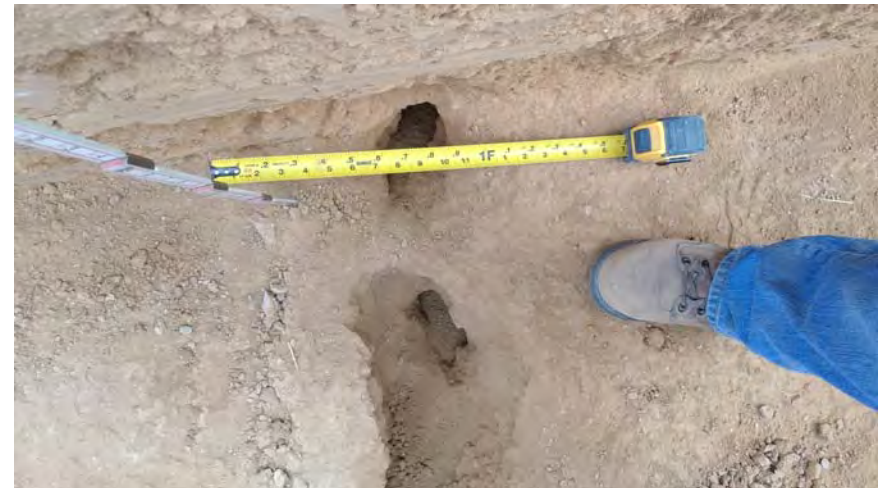
Photo 3: Another view of the eroded fissure crack as it extends into the northwest trench wall.
