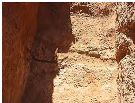
Photo 3: Earth fissure F5 exposed in the bottom of the trench. This photo clearly shows this wide fissure aperture filled with silty, fine to coarse sand crack, that bridges the earth fissure. See Photo 4 that depicts the wide (about 1.4 ft.) filled fissure crack (darker, near vertical soil column) extending upward to the base of the fissure gully fill zone in the east wall of the Trench 3.
