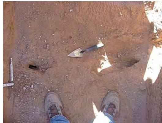
Photo 3: Subsidiary earth fissure-related tension crack (south) about 2 feet south of F4. This crack, with an aperture of about 0.09 ft. to 0.15 ft., was exposed across the bottom of the trench with . This crack opened up into a void a couple of inches below the bottom of the trench. Fissure bearing is N67°W.
