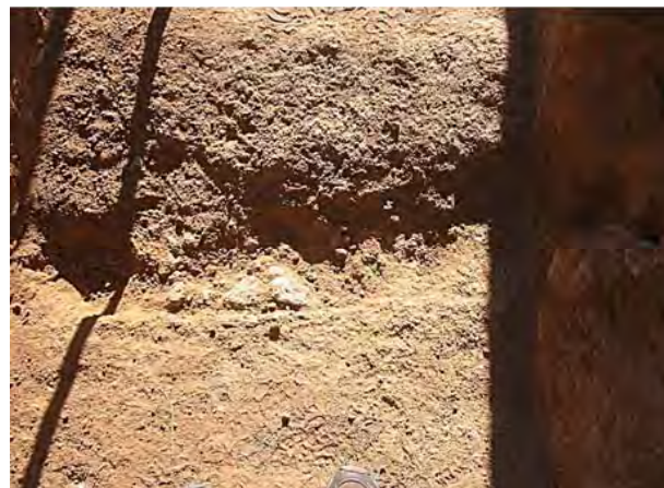
Photo 2: Earth fissure F6 is exposed across the bottom of the trench. The earth fissure crack, about 0.45ft. to 0.9 ft. wide, was found in caliche cemented soil below the overburden soil. The gully fill is with light brown, silty coarse sand mixed with trash and asphaltic concrete rubble. The fissure fill bridges open fissure crack to more than 5 ft. bgs.
