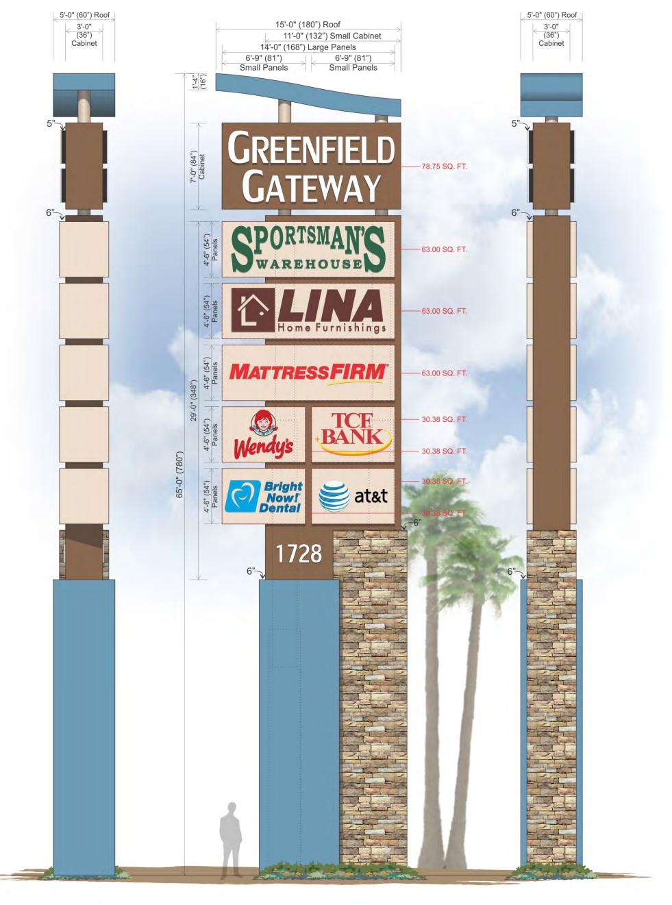
MANUFACTURE AND INSTALL ONE(1) INTERNALLY ILLUMINATED FREEWAY PYLON SIGN SCALE: 3/16" = 1'-0"
