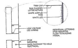
This sign is intended to be installed in accordance with the requirements of article 600 of the national electrical code and/or other applicable local codes. This includes proper grounding and bonding of the sign All signs fabricated as per 2008 N.E.C. Standards
